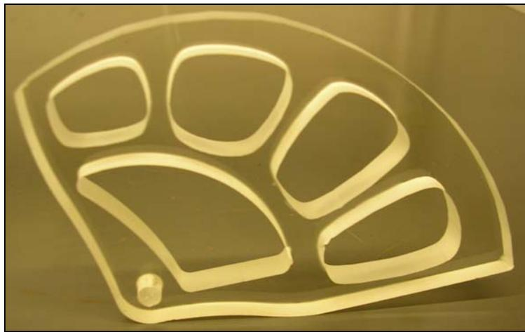
**Figure 6:** Image of Photoelastic model. Made from Homalite H-911 CR-39® plastic sheet.
